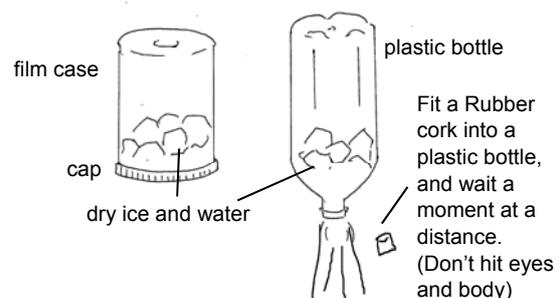
Dry ice rocket is made from a plastic bottle and film case
