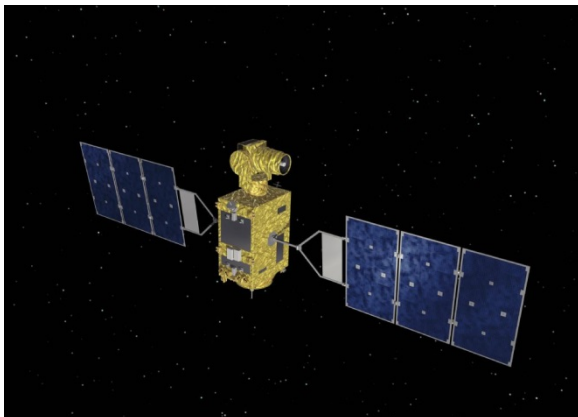
OICETS(KIRARI): Experimental satellite for optical communication between satellites
