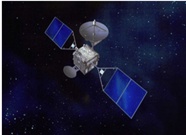
DRTS(KODAMA): Relay technology satellite Communication speed: 240Mbps
