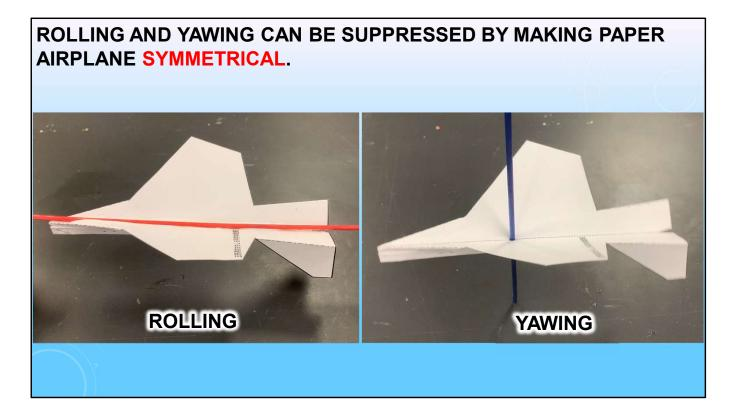
• Rolling and yawing can be suppressed by making paper airplane symmetrical.
