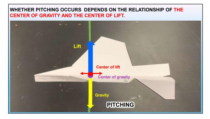
Whether pitching occurs depends on the relationship of the center of gravity, at which gravity acts, and the center of lift, at which lift acts.
