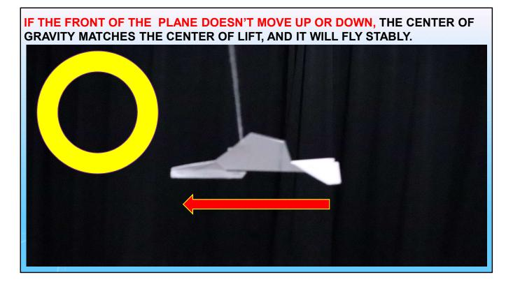
If the front of the plane doesn't move up or down, the center of gravity matches the center of lift, and it will fly stably.
