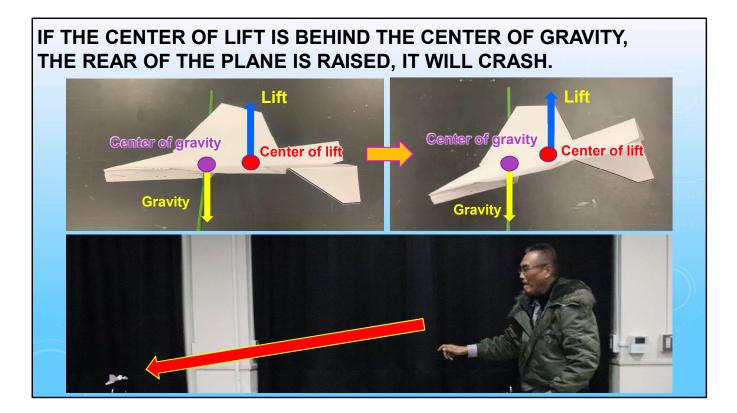
If the center of lift is behind the center of gravity, the rear of the airplane is raised, and it will crash.
